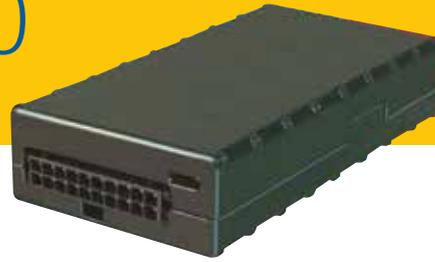
The Sure-Track ST2700 is an extremely sophisticated wired-in fleet management system that has been designed to allow the user to monitor and report on vehicles & machines.
